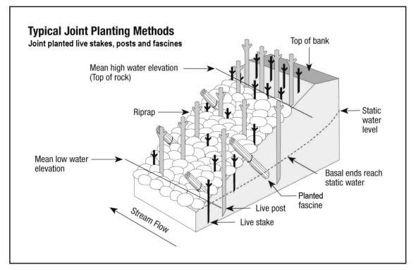
Figure 1. Conceptual drawing of joint plantings to reduce stream bank erosion (B.C. Ministry of Environment, Lands, and Parks and Ministry of Forestry, 1997).
